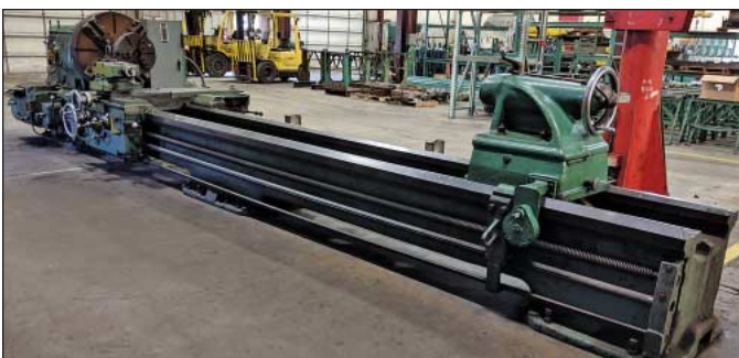
40" x 19' Monarch Model 32" NN Engine Lathe
