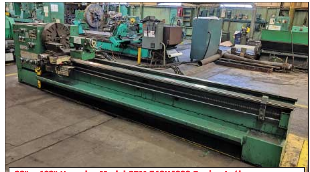
28" x 168" Hercules Model SPM 710X4000 Engine Lathe
