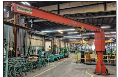
(3) 12' Arm Free-Standing Jib Cranes to 1 Ton by Bushman & Gorbel
