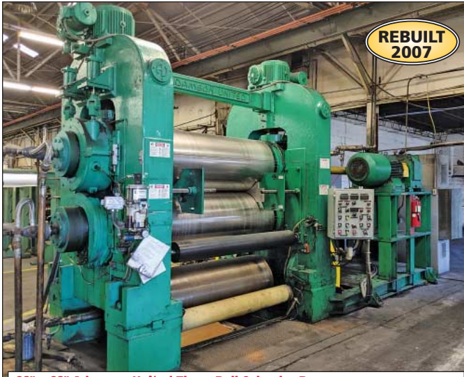
28" x 68" Adamson United Three-Roll Calendar Processor
