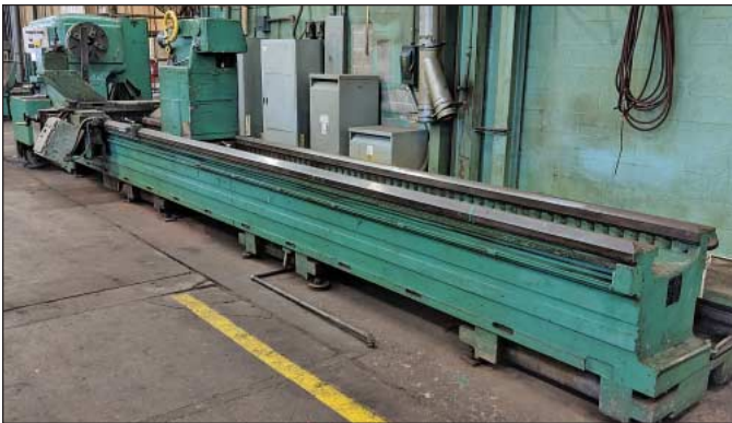
60" x 22' Monarch Engine Lathe
