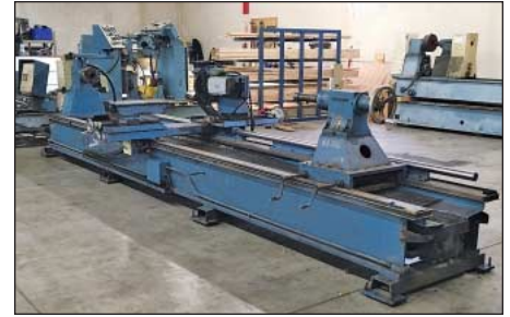
30" x 190" Remco Model GG130x190 Programmable Grinder Groover
