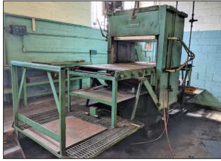
(3) French Oil Heated Platen Compression Molding Presses
