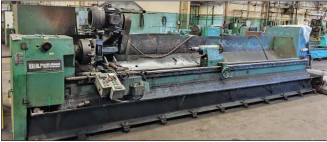
28" x 18' South Bend Roll Grinder
