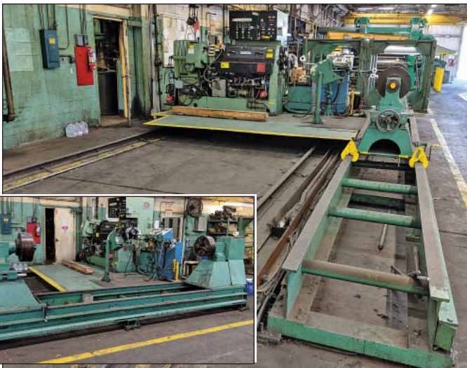
64" X 240" Remco Rollmaster Strip Builder w/3.5" David Standard Rubber Extruder
