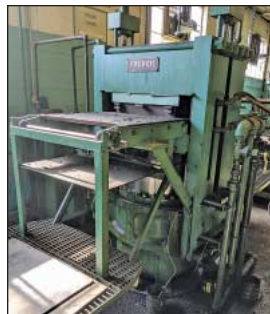
(3) French Oil Heated Platen Compression Molding Presses
