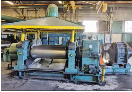
18" x 60" Stewart Bolling Unitized Base Rolling Mill
