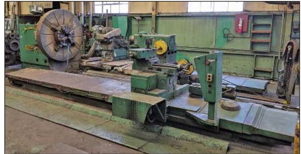
80" x 16' Safop Leonard Model 1500-TR Heavy Duty Lathe w/ Grinding Attachment
