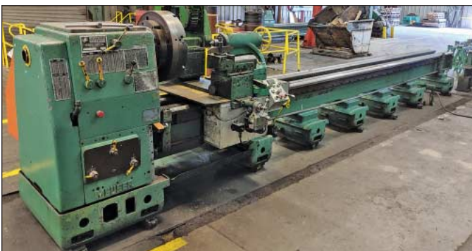
36" x 240" Meuser & Co. Engine Lathe w/ Sander Attachment
